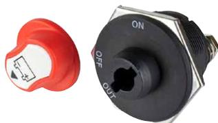
This Battery Switch features a removable knob for extra security. To remove, simply twist the cap to the OUT position and pull. Small footprint makes it ideal for close quarters. 300A continuous and 1000A cranking amps. Constructed of machined brass and injection molded nylon. Installation is as easy as drilling a 1-1/2" hole, inserting the socket body, tightening the locking nut, and connecting the wires.
